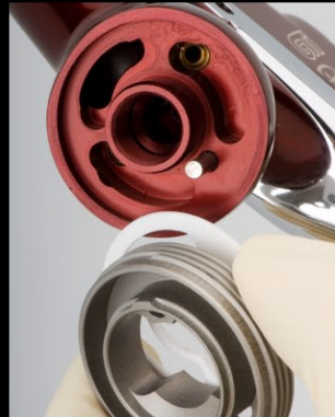
Removing the air separator and seal provides unrestricted access to the front end for easy cleaning.
